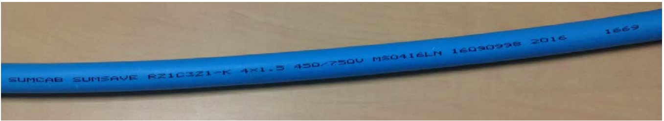
Figure 6.4.5.1 Example of ITER cable jacketing marking, with the manufacturer's name and product reference, number and size of conductors, rated voltage, ITER type code, manufacturer's traceability, year of manufacture and sequential length. The blue jacket identifies the control cables.
