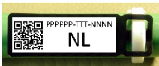
Figure 6.4.3.1 Example of label at the cable extremity
